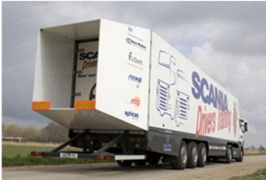
Boat tail reduces truck fuel consumption by 7.5 percent - Source
