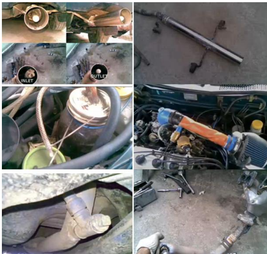
Mr "X's" multiple retro fitting of water injection, hydroxy and the GEET on his Nissan Sentra prototype
